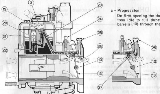
On first opening the throttles (13), that is, when passing from idle to full throttle, mixture also reaches the two barrels (10) through the progression holes (27),
